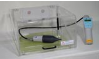
ESD3000 with remote DM for testing explosive devices
